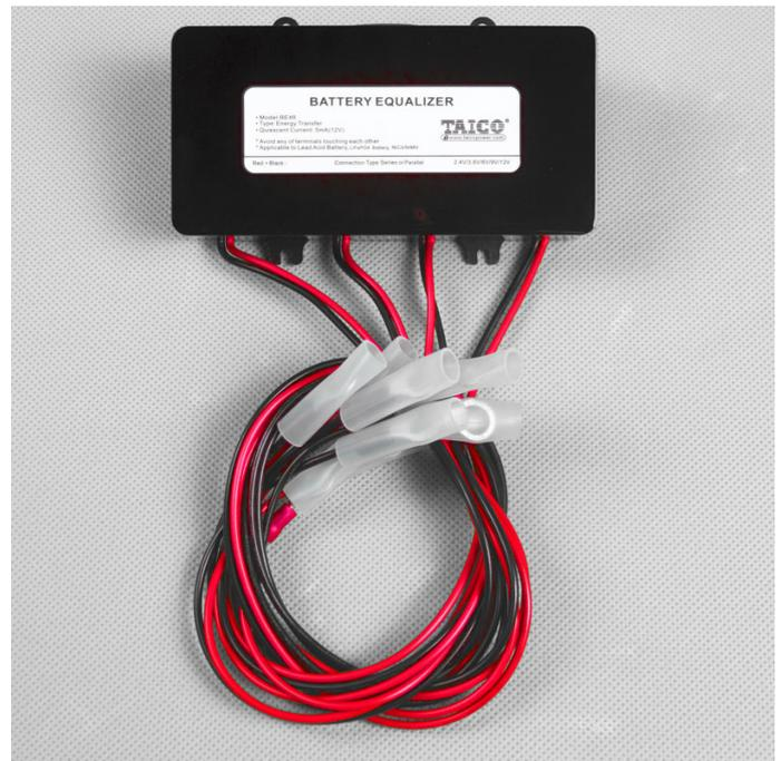
BE48 battery equalizer is energy transfer type equalizer, it can compensate for batteries with two sides. The equalizer starts to work when there are 10mV between two batteries. The current will flow from a higher voltage to low voltage, eventually reach equilibrium. It can connect with battery system with 24 hours, to keep the system energy balance automatically, no need manual maintenance.
